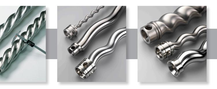
For our standard rotors we use stainless steel 1.4571 or AISI 316 Ti as well as tool steel 1.2436 vacuum-hardened to 61 HRC. Of course we also work with other materials if required.
